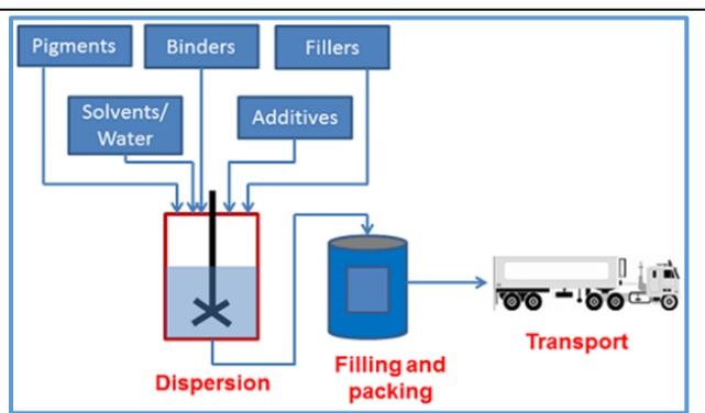
**Figure 1 - Simplified process diagram for architectural coatings manufacturing**
